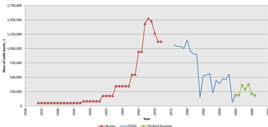
**Fig. 4.** Colliery waste disposal on the foreshore at Lynemouth from 1934 to the closure of Ellington Colliery in 2005. Data are from [Nunny \(1978\)](#) for 1934 – 1972, the Centre for Environment, Fisheries and Aquaculture Science (CEFAS, unpublished data, see ‘Acknowledgements and Funding’ section) for 1976 – 1994, and [Posford Duvivier \(2001\)](#) for 1995–August 2001. Note that data are missing for the periods 1973 – 1975 and 2002 – 2005.
