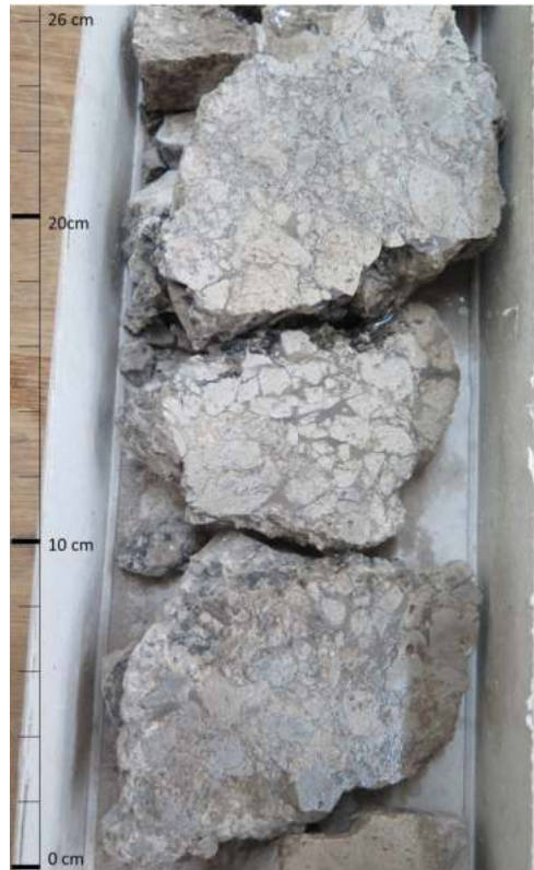
Fig. 20. Core photo taken from the collapse brecciated Argyll Field well 30/24-20 at c. 9801 m depth. The breccia has a clast-supported fabric with angular to subangular clasts, variable amounts of vuggy porosity and shows no sorting; the matrix comprises fine carbonate with variable amounts of clay. Photo based upon sample supplied under loan number: Core 225416 from well 30/24-20 BGS © UKRI.
