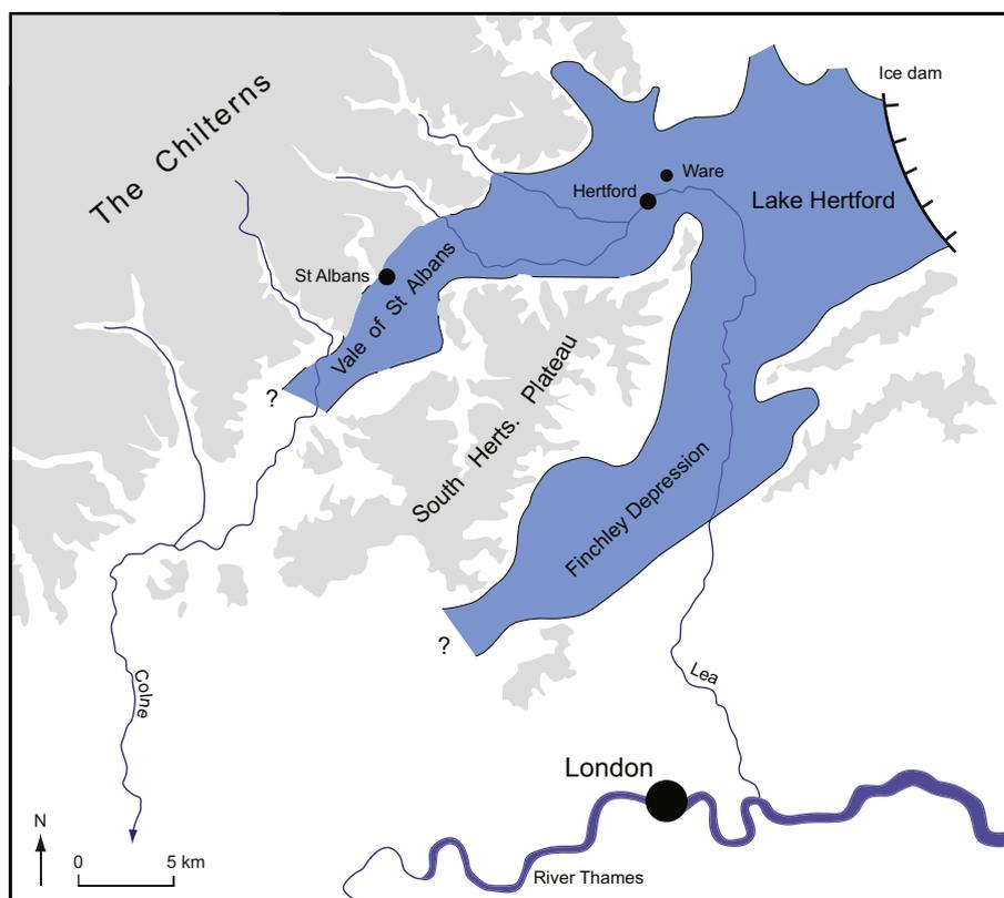
**Fig. 6.** The maximum extent of glacial Lake Hertford and its postulated ice dam during MIS 12. The rivers are shown in their contemporary courses. Contour at 90 m OD. Adapted from Clayton and Brown (1958).
