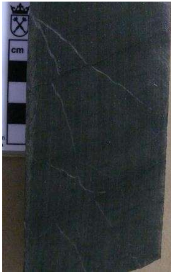
Z2 Slope facies, depth 2590 m. Polish sub-basin. Fractures: some filled, some open, some offset, brecciated zone + vugs.
