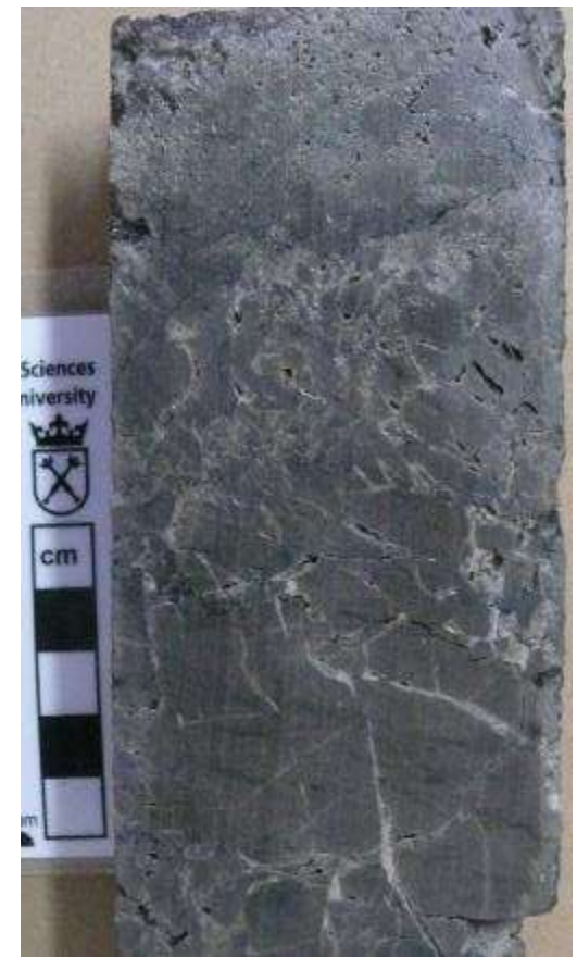
Z2 Slope facies, depth 2590 m. Polish sub-basin. Fractures: some filled, some open, some offset, brecciated zone + vugs.
