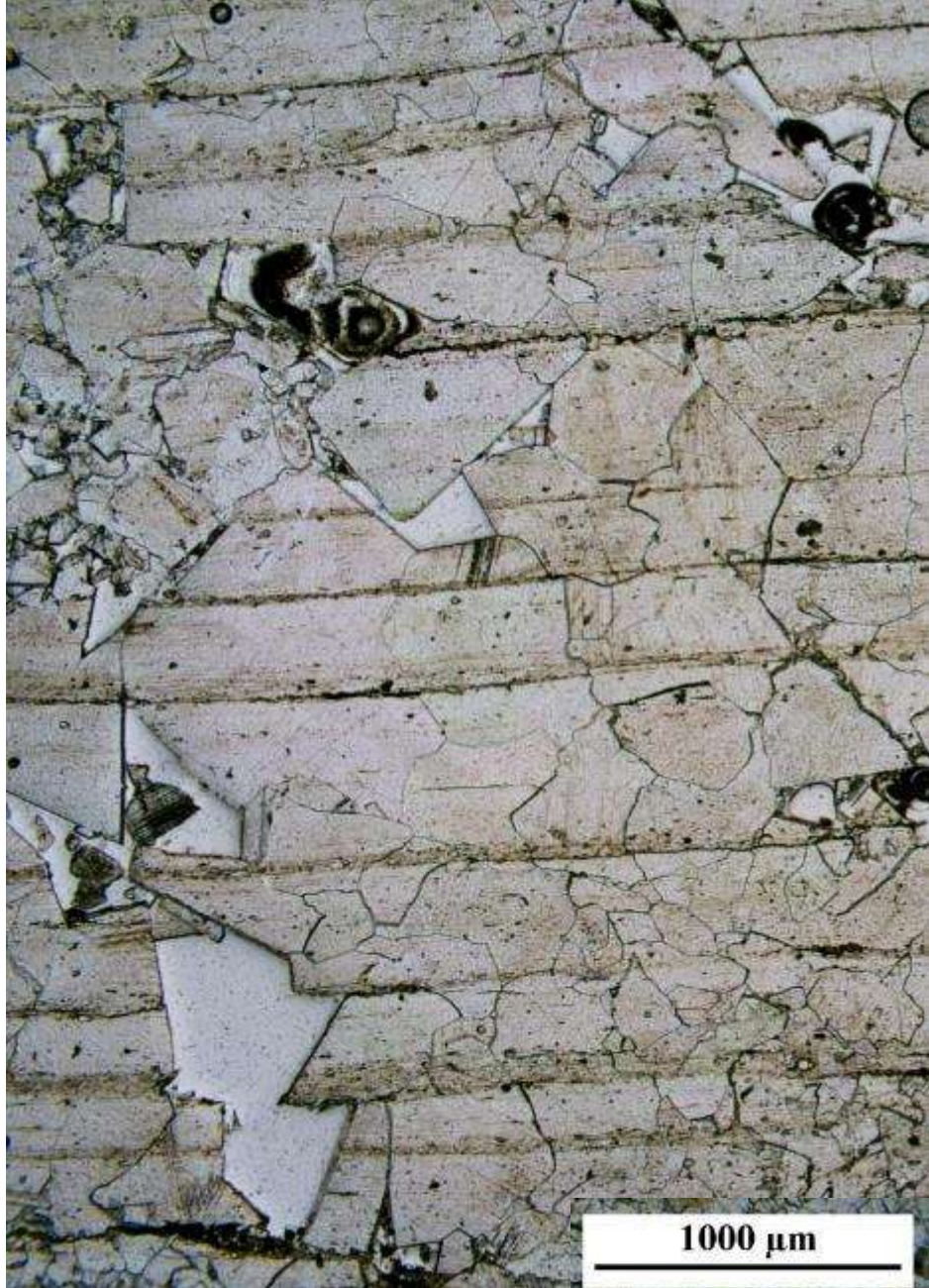
Calcitised slope laminites, Roker Fm., NE England. PPL & XP. \delta^{13}\text{C} = 5.8 \text{ ‰} , \delta^{18}\text{O} = -4.0 \text{ ‰} . Secondary limestone - dedolomite
