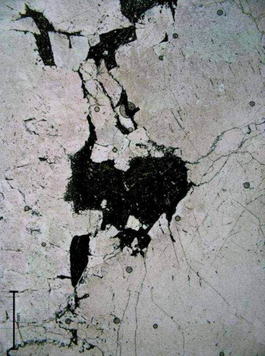
Hydrothermal – deep burial dolomite + bitumen. Scale bar = 1 mm. Lockton-2a: saddle /baroque dolomite. Isotopes: \delta^{13}\text{C} 4.2 ‰, \delta^{18}\text{O} -13.95 ‰.
