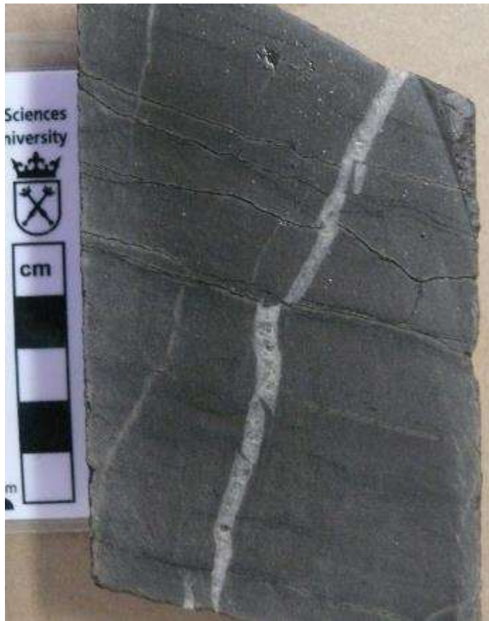
Z2 Slope facies, depth 2590 m. Polish sub-basin. Fractures: some filled, some open, some offset, brecciated zone + vugs.
